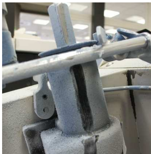
Rewinding machine: without the use of FIBERMATE POC
